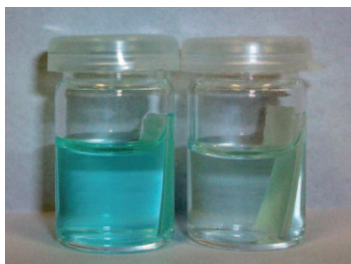
Figure 4. Photograph of a 1 × 2 cm silica dipstick immersed in a solution of SD ( 2.6 \times 10^{-6} M) in acetonitrile. The left-hand foil was previously exposed to air that contained 5 ppm DFP, whereas the right-hand foil was directly dipped into the SD solution.
